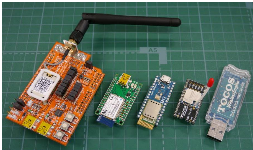
xPicoWiFi、RN42、mbed HRM1017、TWE-Lite DIP、ToCoStick (WiFi) (Bluetooth)(BluetoothLE) (IEEE802.15.4)
